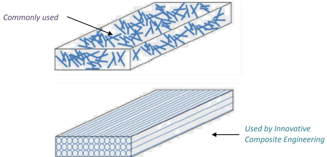
Innovative Composite Engineering uses continues fibers, which have much superior load bearing properties. We engineer each product to know the exact loads and forces acting on the part and thus engineer the fiber orientation accordingly. This needs a complete stress analysis of the part and a much advanced manufacturing technique.
