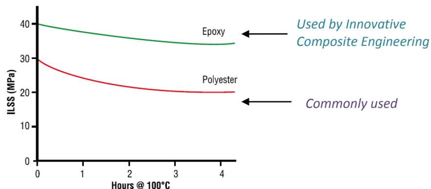
! - Effect of Periods of Water Soak at 100°C on Resin Inter-Laminar Shear Strength
